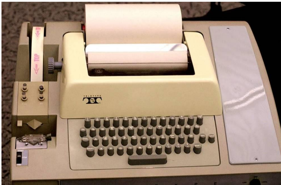
Figure 32 – Refurbished ASR-33 Teletype (B.Blackburn 2009) (On left side, back to front: Blank roll of paper tape, Punch unit, Reader unit.)
