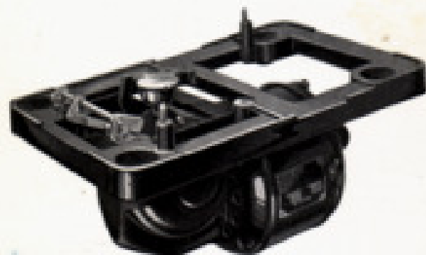
THE MOTOR DRIVE UNIT
