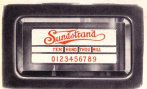
In correcting with the error key, the digit indicator is helpful because you can see the arrow move along to the left (toward zero) as you take out the units one at a time with the error key.
