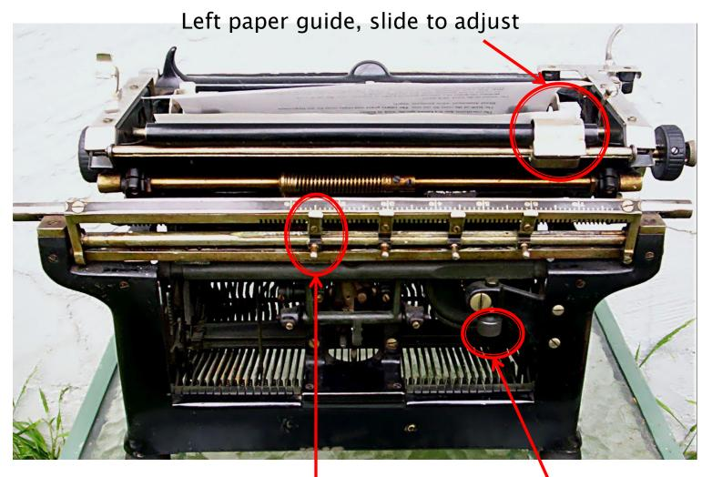
Rotate tab-stops out of grooves, slide to new position, rotate back securely into gear-like grooves
